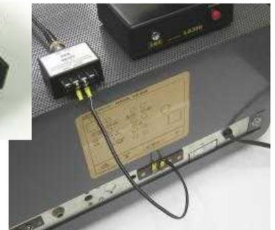
MC-600 is an optional interface between the 600Ω antenna socket of your antique radio, and the 50Ω input of the LA390 (or LA380) loop antenna. Supplied with a 30cm lead terminated with solderless terminals.
