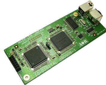
**GPS receiver – GP5001:** Improves the frequency stability of AR6000 from  $\pm 0.1$ ppm to  $\pm 0.01$ ppm, by using the GPS pulse signal for an accurate time base of the local oscillator circuit.
