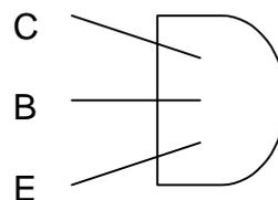
Note; The BC327 fits the board as per the layout, the J310 Gate has to be positioned to the centre pin.
