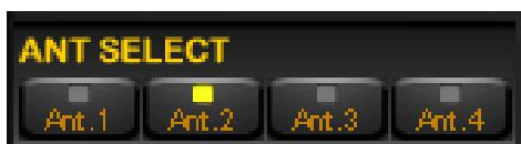
Ant.3 and Ant.4 do only function if the receiver is AR5001D and the optional AS5001 antenna selector is used.
