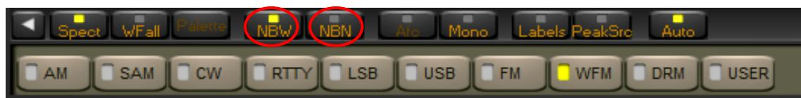
The Narrow NB, operates on the bandwidth selected with the BW buttons (56 kHz, 28 kHz, 14 kHz, etc).
