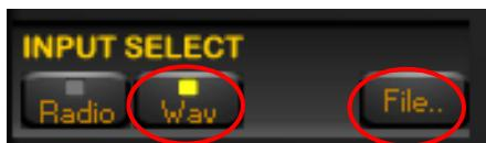
The receiver stops receiving live signals and the "Wav" and "File" buttons are now activated. Click "File" and browse on the PC to the location of the pre-recorded file(s). Then simply press the PLAY button (button with white triangle).
