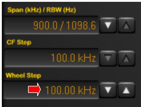
This is the value by which the spectrum will be shifted by scrolling the mouse wheel, when the mouse is hovered anywhere over the spectrum or waterfall.
