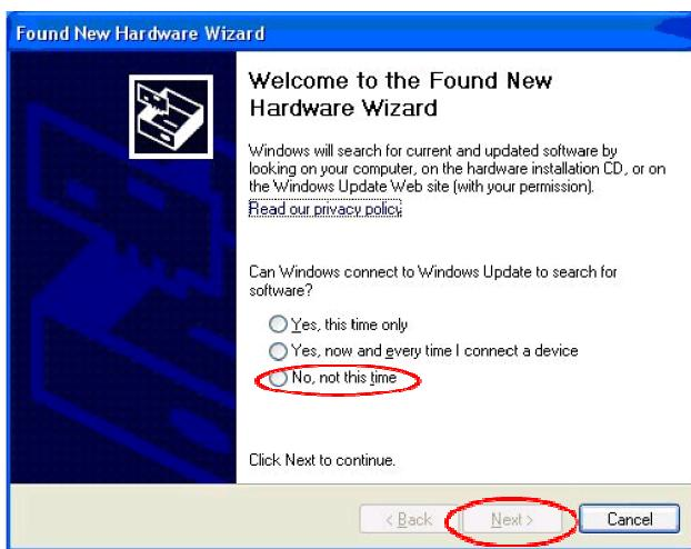
**64bit:** Windows although detecting the USB connection, will fail to automatically install the I/Q driver. You will need to install it manually as follows:
