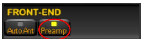
Switches the receiver's front-end pre-amplification on. When in the ON position, the attenuator level is set to 0dB.
