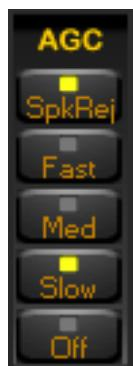
The Automatic Gain Control keeps the audio output at a constant output level, disregarding the input signal power. Three time decay constants can be selected with the buttons “Fast”, “Med”, and “Low” in the AGC control bar.
