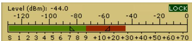
functions. Squelch level can be enabled clicking the bar in the S1-S9 (green) zone with the left mouse button; any signal under the set
