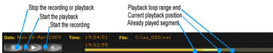
I/Q recording takes about 700MB of disk space per minute, which is 42GB per hour, or 1TB for 24 hours. Make sure you have plenty of disk space available depending of the desired length of the recording.
