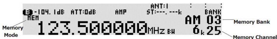
If more than one memory channel is programmed into the current memory bank, and when an ‘active’ channel has been located (busy, so the squelch opens), the scan process will temporarily pause on the active channel. The memory location (such as “25”) will be displayed along with any accompanying text.
