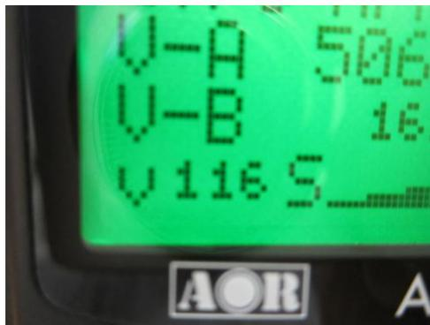
5. Rotate the squelch knob counterclockwise to display “S” icon on the center bottom of the LCD. The background squelch noise will be heard.
