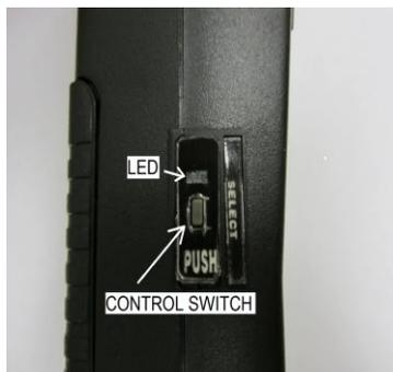
4. To stop recording, press and hold the **[CONTROL]** switch again for two seconds. The red LED will go off.
