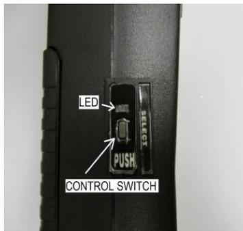
2. Double clicking the **[CONTROL]** switch will toggle through the APCO25 mode (one beep), Voice Inverter mode (two beeps), and CTCSS mode (three beeps).
