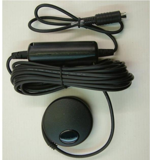
The GP5001 GPS receiver system differs from typical “map based” positional systems. It feeds a highly accurate one-pulse-per-second (PPS) signal to the AR2300/AR5001D receiver. The rising edge of the signal is aligned to the start of each GPS second within 1µsec.
