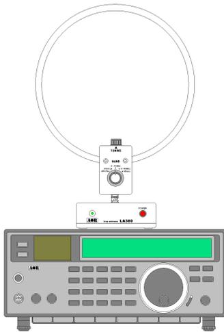
The **LA380** is a compact active (30cm diameter) loop aerial specifically designed to provide good reception when away from the main monitoring location or when large external aerials are not practical. Compact, but achieving high performance, featuring an internal high-gain amplifier (20dB for 10kHz-250MHz) and excellent overall strong signal handling (high IP3 +10dBm).
