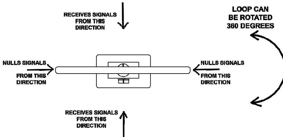
A rotating loop antenna is very directional. The loop will allow signals on opposite sides to be received, while off the sides of the loop the signal will decrease or be nulled out.
