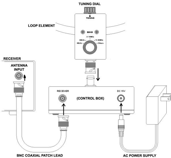
1) Connect the power supply to the rear panel DC input socket, the LA380 requires 12V DC at 50mA (9-15V DC). A 9V regulator is built into the LA380 control unit. To minimize noise, keep the power supply as far away from the LA380 as practical. To minimize electrical interference from the power supply, for the receiving range between 10kHz and 1.6MHz, you may wish to consider use of a (non supplied) low noise regulated power supply.
