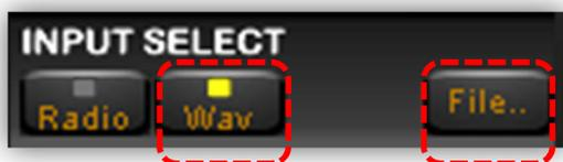
The receiver stops receiving live signals and the "Wav" and "File" buttons are now activated. Click "File" and browse on the PC to the location of the pre-recorded file(s).
