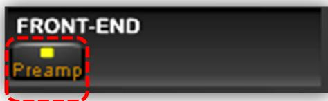
Switches the receiver's front-end pre-amplification on. When in the ON position, the attenuator level is set to 0dB.
