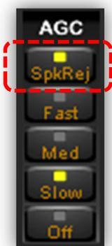
The Spike Rejection function emulates the behavior of the AGC of old analog receivers with a relatively long attach time constant. When this function is selected the AGC circuit is much less sensitive to impulse noise which can completely close the receiver gain and affect negatively the receiver performance.
