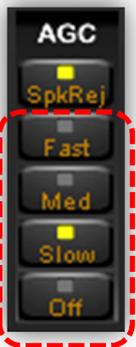
The Automatic Gain Control keeps the audio output at a constant output level, disregarding the input signal power. Three time decay constants can be selected with the buttons “Fast”, “Med”, and “Low” in the AGC control bar.
