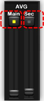
**AVG Main:** Stabilizes the spectrum waveform in the main spectrum / waterfall display. Will also stabilize the waterfall mode. The main spectrum average function and its slider control are active only when the enable button above the slider is enabled.
