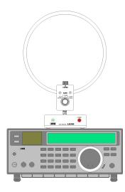
The **LA380** is a compact active (30cm diameter) loop aerial specifically designed to provide good reception when away from the main monitoring location or when large external aerials are not practical. Compact, but achieving high performance, featuring an internal high-gain amplifier (20dB for 10kHz-250MHz) and excellent overall strong signal handling (high IP3 +10dBm).
