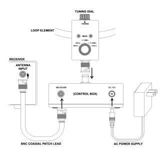
1) Connect the power supply to the rear panel DC input socket, the LA380 requires 12V DC at 50mA (9-15V DC). A 9V regulator is built into the LA380 control unit. To minimize noise, keep the power supply as far away from the LA380 as practical. To minimize electrical interference from the power supply, for the receiving range between 10kHz and 1.6MHz, you may wish to consider use of a (non supplied) low noise regulated power supply.
